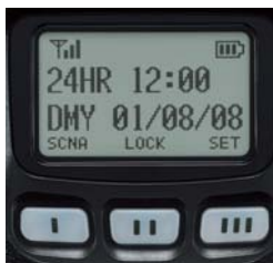
Internal clock setting example
